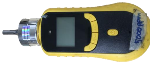
FIGURE 3-5 ozone detector SKZ-1050-O 3
