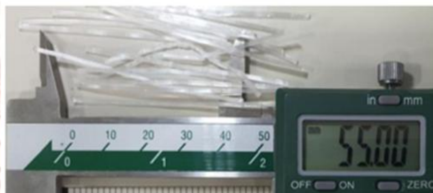
Figure 27 Polypropylene Fiber lengths of 55 mm
