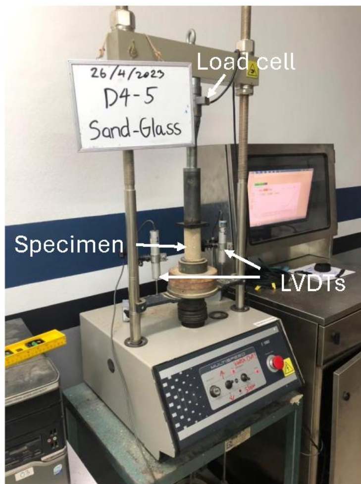
Fig. 7. Unconfined compression test set-up.
