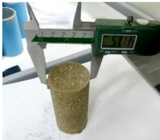
Fig. 5. Measurement of specimen diameter.
